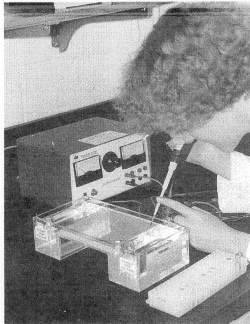
Figure 12.3 A scientist is using a micropipette to load DNA sample into an agarose gel. The gel is in an electrophoresis chamber full of buffer. The power supply for the chamber is on the laboratory bench behind the chamber.
